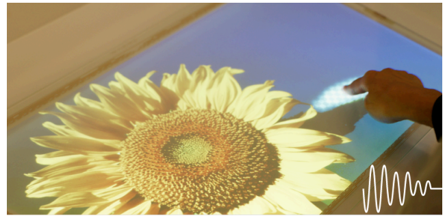
Figure 14: Friction between a user's finger and the touch surface decreases as the user increasingly erases a projected image by rubbing it.
