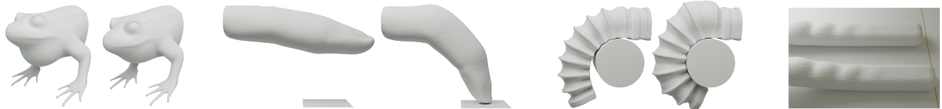
Figure 1: Shape optimization of a pressure cavity. We optimize the interior cavity of pressurized chambers to reach prescribed shapes (Frog, Finger, Gripper), displacements (Worm), and contact forces (Gripper). These results are then fabricated and tested experimentally to validate the efficacy of our pipeline.
