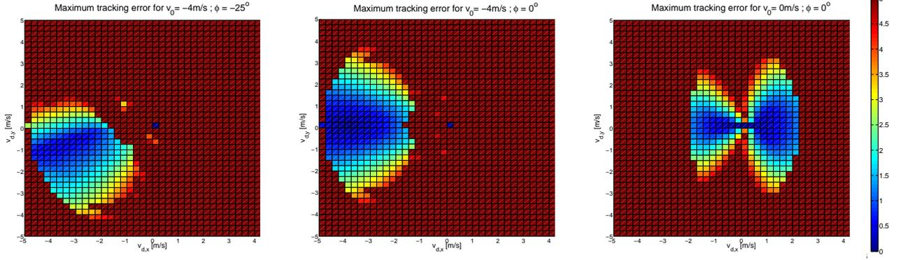
Fig. 2. Maximum tracking errors in  $[m]$  for a desired trajectory given by  $\mathbf{v}_d \in \mathcal{V}$  and saturated at 5m. From left to right, the initial driving velocity  $v_0$  and the steering angle  $\phi$  vary from  $(v_0, \phi) = (-4\text{m/s}, -25^\circ), (-4\text{m/s}, 0^\circ)$  to  $(0\text{m/s}, 0^\circ)$ . Images best viewed in color.
