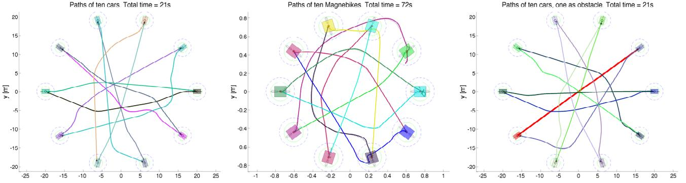
Fig. 5. Trajectories of ten car-like robots exchanging antipodal positions on a circle. **Left:** Experiment 1 with car-like vehicles. **Middle:** Experiment 1 with MagneBikes. **Right:** Experiment 2, where one car is non-reactive (straight-line trajectory in red), thus ignoring the other robots.
