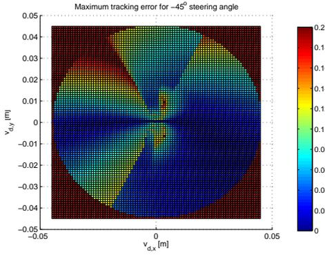
Fig. 3. Maximum tracking errors in [m] for a desired trajectory given by  $\mathbf{v}_d \in \mathcal{V}$ , here shown for  $\phi = -45^\circ$ . In the case of MagneBike,  $v_0$  is set to  $s_1 v_d$ , and thus precomputation includes varying steering angles only.
