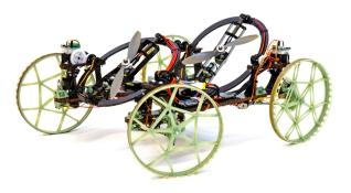
The robot is able to move on a wall quickly and with agility. The use of propellers to provide thrust onto the wall ensures that the robot is able to traverse over indentations such as masonry. The choice of two propellers rather than one enables a floor-to-wall transition - thrust is applied both towards the wall using the rear propeller, and in an upward direction using the front propeller, resulting in a flip onto the wall.
