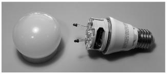
Figure 7: Assembled smart LED light bulb with unscrewed cap and connected phototransistors.
