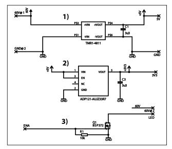
Figure 4: Schematics of the dedicated power module PCB. 1) DC/DC power converter, 2) 3.3 V regulator, 3) N-channel MOSFET.
