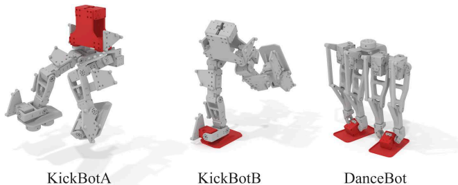
Fig. 4. The robots. KickBotA (attached at the pelvis), KickBotB (attached at the right foot), and DanceBot (attached at both feet). Fixed components are shown in red.
