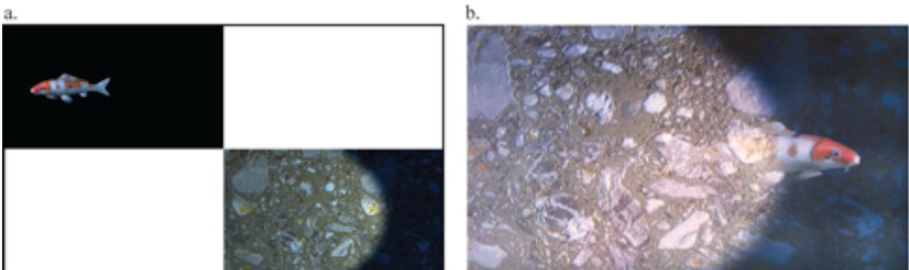
Figure 9a. Double-wide over-under image format for switching Dual Layer Display with Mask with front layer content (upper left), front mask (lower left), and background content (lower right). Left frames displayed on front transparent LCD panel; right frames displayed on rear LCD monitor. b. Image from the Switching Dual Layer Display with Mask, alternating
