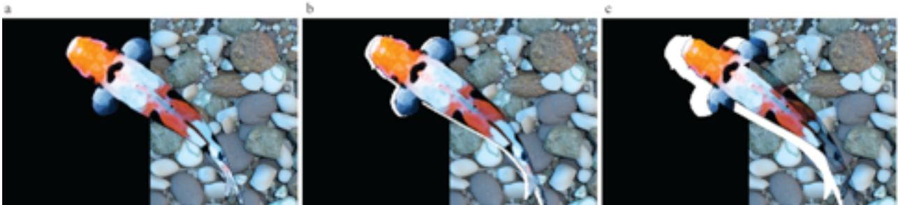
Figure 2a. Pure Depth's Multilayer Display makes the front layer content visible and apparently opaque (when viewed on-axis) by aligning front layer content with a matching white silhouette on the back layer. b. A halo appears when viewed slightly off-axis due to parallax between layers. c. White silhouette apparent when viewed off-axis.
