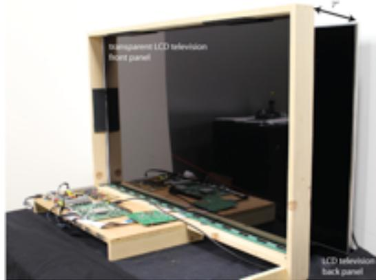
Figure 6. A Switching Dual Layer Display using two stacked and spaced 55" LCD televisions.
