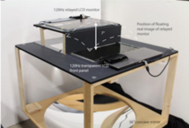
Figure 11. A tabletop Floating Switching Dual Layer Display using a 36” diameter, 15” FL concave mirror and two 23-inch 120Hz monitors. The mirror relays an image of the relayed monitor so it floats above the transparent monitor.
