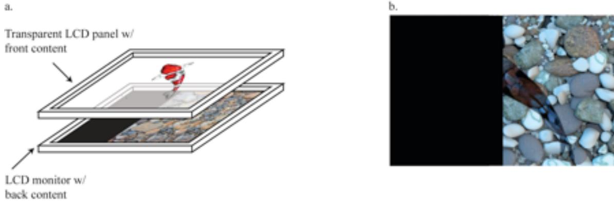
Figure 1a. A basic dual layer display using a transparent LCD panel stacked and spaced over a LCD monitor.
