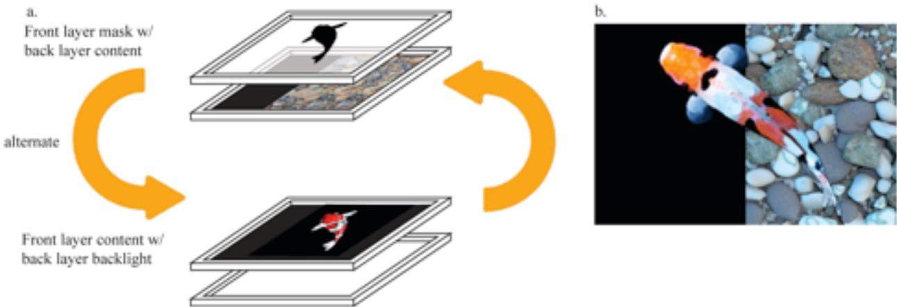
Figure 4a. A Switching Dual Layer Display with a Dynamic Mask alternates between front layer content with back layer backlight, and front layer mask with back layer content. b. Front layer is independent of back layer content. Front content appears over dark background content (left), and front layer content appears opaque and high-contrast over bright background content (right).
