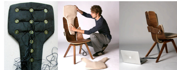
figure 4. A haptic display, a pattern of vibrating transducers arranged in a pattern in a pad, is mounted on the custom made gaming chair.
