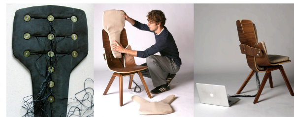
Figure 2. Modular tactile gaming platform (a) pad with tactile actuator grid (b) assembling gaming chair (c) home tactile gaming setup.
