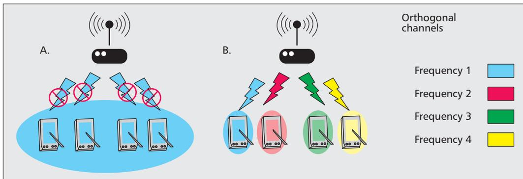
**Figure 4.** Devices operating on orthogonal channels do not interfere.
