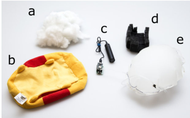
Fig. 4. Pressure data transmitting doll components including (a) stuffing, (b) fabric covering with zipper, (c) 3350 mAh battery, pressure sensor and Wi-Fi enabled microcontroller, (d) foam microcontroller housing and (e) heat-sealed polyurethane air bladder.
