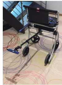
Fig. 5: Experimental setup - an Intel RealSense ZR300 mounted on a manually pushed trolley.
