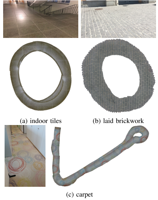
Fig. 8: Map mosaics for indoor tiles, laid brickwork, and carpet. The diameters of the circular trajectories are about 3m, and the full length of the trajectory on carpet is about 7m. Qualitative evaluation can be done by zooming on the tile or brickwork mosaics to inspect the rectilinearity of lines.
