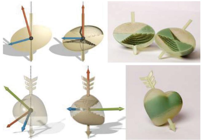
**Figure 5. “Break-dancing Armadillos”:** Through our hollowing optimization, the Armadillos can perform spinning dance moves. For each design, the unstable input (left), and the optimized stable output (right) are shown. The Armadillo on its shell is particularly badly aligned in the initial model.
