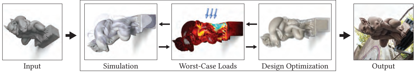
Fig. 2. Overview. As input, our optimization takes a 3D model, parameterized loads, grounded surface regions, and a design space (Input). To optimize the strength-to-weight ratio, we first solve for the loads that maximize the potential of failure (Worst-Case Loads) under static equilibrium constraints (Simulation). We then minimize the potential of failure under these worst-case loads (Design Optimization), adding objectives to reduce weight and place the center of mass. To unify all three stages into a continuous optimization, we enforce first-optimality of our worst-case load estimation and simulation when solving our design optimization. Our output structure is sound and withstands worst-case loads drawn from a subspace of uncertainty (Output).
