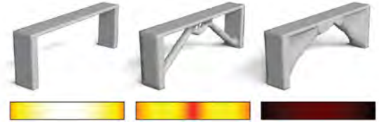
Fig. 14. Failure Objective Energy Landscape We show the energy landscape (bottom) of the objective f_{\text{fail}} for all positions of a load applied to the top surface of the bridge. For an unoptimized bridge (left), the load location that leads to the highest energy—the location of the worst-case load—is in the center. For the fixed-load optimized bridge (center), the locations for the worst-case loads move to the two ends, and the effect of these loads is weaker. The bridge optimized under worst-case loads (right) no longer has any load locations that would lead to failure.
