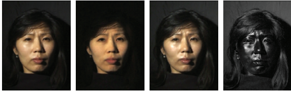
Figure 5: Diffuse-specular separation using polarization [DHT*00], from left to right: reference image without polarizers; cross-polarization yields diffuse reflectance only, parallel-polarization yields diffuse and specular reflectance, subtracting the cross-polarization image from the parallel-image yields the specular reflectance only.
