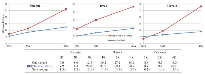
**Table 2:** Timings for computing scattering using our method and the method of Billeter et al. [2010] on versions of our scenes with a spotlight instead of a directional light. The timings for each scene are for three shadow map resolutions and are given in milliseconds. For the terrain scene at 4K resolution, we used the adaptive version of Billeter et al.'s method because it was 1.8ms faster than the non-adaptive version.
