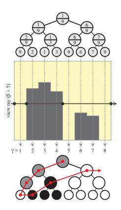
**Figure 4:** The min-max mipmap (top) corresponding to a row of the rectified shadow map in the scene from Figure 1. To compute the scattering integral for any view ray in this epipolar slice (middle), we traverse the tree by thresholding the min-max mipmap with the  $\beta$  value of the view ray (bottom). Nodes entirely in shadow are colored black, nodes entirely lit are colored white, and nodes containing visibility boundaries are grey.
