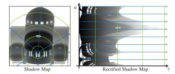
**Figure 3:** We perform rectification on the shadow map (left). This turns epipolar slices (radial lines emanating from the epipole, left) into rows of our rectified shadow map (right). For this directional light, the radial distance from the epipole is the coordinate  $\gamma$  which specifies a column within each slice. The value of each pixel in the rectified shadow map gives the  $\beta$  coordinate of the occluder.
