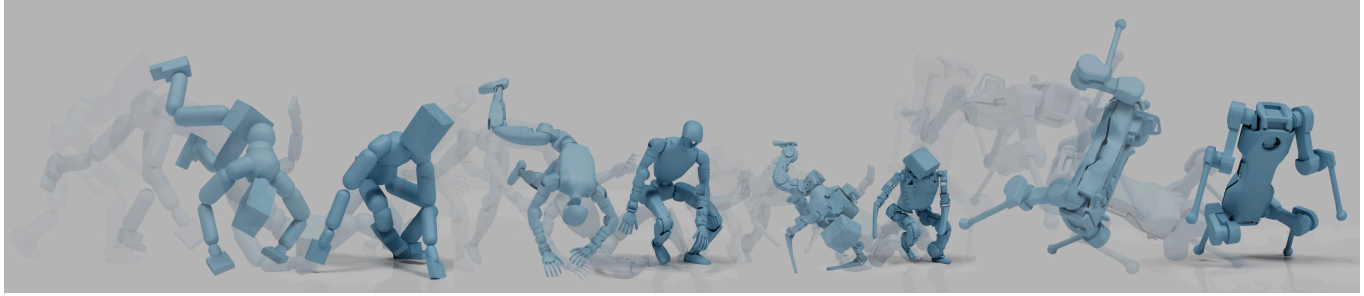
Fig. 1. Physics-aware retargeting of human motion (left) onto two humanoid robots (middle) and a quadruped (right) with varying degrees of freedom and vastly different shapes, sizes, and proportions.
