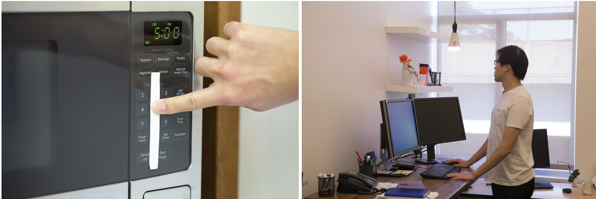
Fig. 12. In this interaction, a user presses the quick-cook button on a microwave augmented with a touch sensitive tag. An RFID lightbulb in the user’s office flashes to notify the user of the microwave timer has expired.
