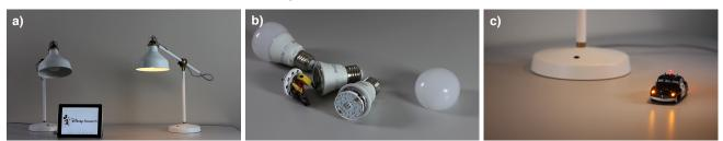
Figure 1. a) Demo setup with off-the-shelf lamps, b) modified consumer light bulbs, c) toy car equipped with VLC technology
