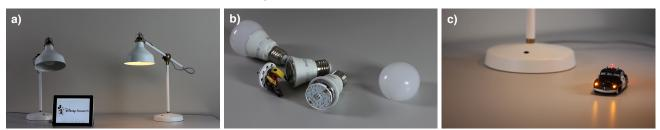
**Figure 1.** *a)* Demo setup with off-the-shelf lamps, b) modified consumer light bulbs, c) toy car equipped with VLC technology
