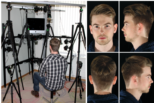
Figure 4: Our capture setup consists of 10 cameras placed in a quarter-sphere and we capture 4 different orientations of the subject.
