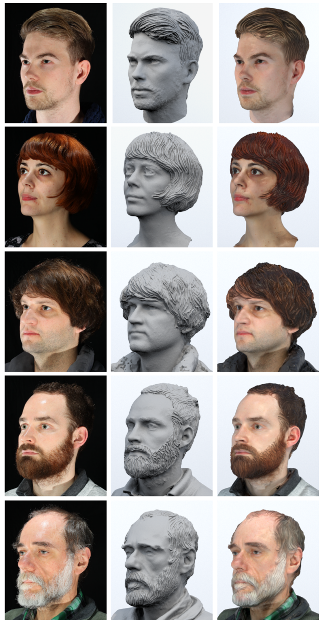
Figure 13: Our stylized hair capture technique can reconstruct a wide range of hair-styles, including the facial hair on the subjects in the bottom two rows. Here we show one of the input images (left), the stylized geometry without color (center), and the final result with stylized shape and color (right).
