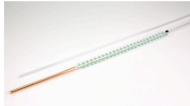
Figure 2. Acrylic rods: a bare rod and a rod with LEDs, conductive tip (copper) and wiring.
