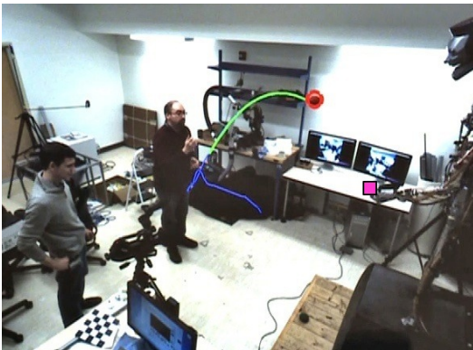
Fig. 3. Each camera performs ball detection (red circle) independently. The 3D coordinate of the ball (blue curve) is then triangulated from the pair of 2D image locations. When a throw is detected, a Kalman filter (green curve) processes the raw 3D positions and predicts a 3D catching location (pink square) and time to impact.
