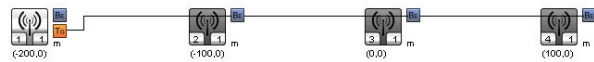
Figure 5. The line scenarios with a single data stream from Station 1 to Station 4. The distance between two neighboring stations is 100m.
