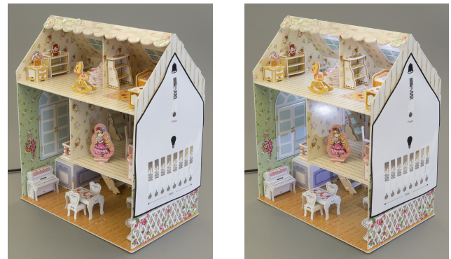
Figure 11. Paper interfaces can be used to create new sensors to control the lighting and doorbell of this foam doll house.
