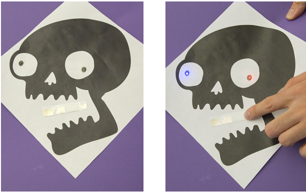
Figure 13. Using the same antenna with which we sense our input tags, we can wirelessly power LEDs. We are using a single touch tag as our input to increase or decrease the reader's power output.
