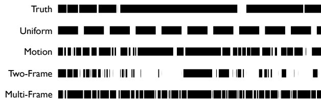
Figure 8. Summarization Visualization. The subset of frames \mathcal{F} selected by each method to include in the summary are shown in white. The two-frame tracking method is able to recall all ground truth events of interest, but generates a very long summary video. The multi-frame tracking algorithm generates the most concise summary, while maintaining a fairly high recall.
