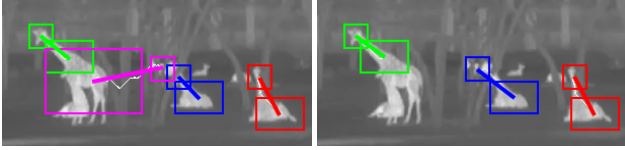
Figure 6. Greedy vs Linear Assignment. Head-body associations made in a greedy fashion using Euclidean distance can easily lead to incorrect solutions (left). The geodesic distance (right), in combination with a linear assignment formulation, significantly improves the correct association of heads to bodies.
