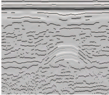
Figure 2. Processed B-Scan with WORMs extracted and classified. Whiter lines are predicted to be potential nest WORMs, and darker lines correspond to predicted background WORMs.
