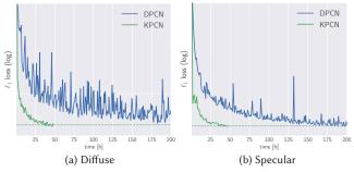
Fig. 9. Comparison of optimization speed between the DPCN and KPCN architectures. Although both approaches converge to a similar error on the *Cars 3* validation set, the KPCN system converges 5–6× faster.
