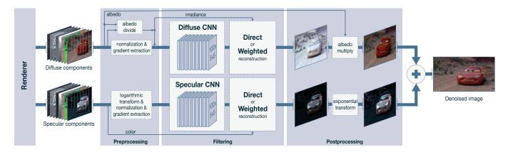
Fig. 2. An overview of our general framework. We start by preprocessing diffuse and specular data coming from the rendering system independently, and then feed the information to two separate networks which denoise the diffuse and specular illumination, respectively. The output from each network undergoes reconstruction and postprocessing before being combined to obtain the final, denoised image.
