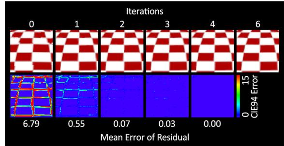
Figure 9: The result and residual error after each iteration for a curved patch on the sphere.
