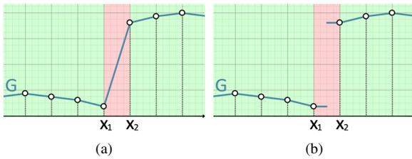
Figure 4: Adaptive sampling in the presence of a steep gradient/discontinuity (shaded red). Using naive interpolation results in the reconstruction in (a). The convergence term (equivalent to  $|G'(x)|$  in 1D) is greater than 1 between  $x_1$  and  $x_2$ , violating the convergence condition (Equation 8), and FPI will not converge to any solution in this region. Switching to point sampling (b) extrapolates the signal into the discontinuity.
