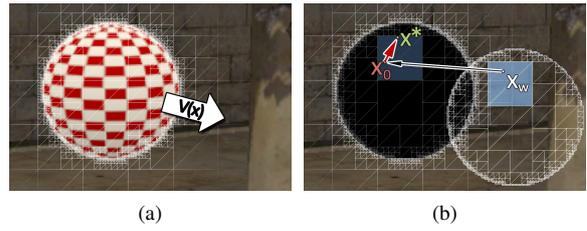
Figure 5: Robust iterative warp. The source image is recursively subdivided until no quad straddles a discontinuity in the warp field (a). To perform the reprojection, the quads are rasterized at their warped locations (b). The iteration starting point  $x_0$  is then interpolated from the quad and used as the starting point of the iteration. The iteration (red arrow in (b)) is guaranteed to converge to the solution  $x^*$ .
