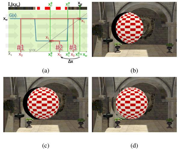
Figure 2: Heuristics-based reprojection. (a) A cobweb plot of some example trajectories at the right hand side of the sphere. (b) When the current pixel coordinates are used as the iteration start point, the behavior resembles trajectory #3 with convergence to solution  $x_2^*$  on the background. (c) The iteration start point is offset  $\delta x$  pixels to the left, starting the iteration on the sphere and yielding the desired solution  $x_0^*$ . (d) Inpainting using surrounding texture.
