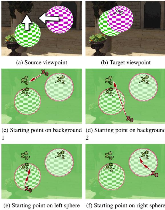
Figure 3: Iteration trajectories (red arrows) for a selection of start points  $x_0$  in an example scene in which (a) is warped forward in time to (b). Each solution  $x_i^*$  indicates a point on a surface in the source view (a) which warps to the target pixel at  $x_w$  in (b). The divergent pixels (shaded red) form boundaries around convergent regions (shaded green), within which convergence to any solution is guaranteed.
