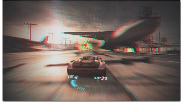
Figure 6: Stereoscopic reprojection with offset heuristics (Section 3.3) fitted as a post process to an existing racing game. The overhead per view is only 0.85ms on Sony PlayStation 3 hardware. For anaglyph both views can be computed in a single pass in under 1ms.
