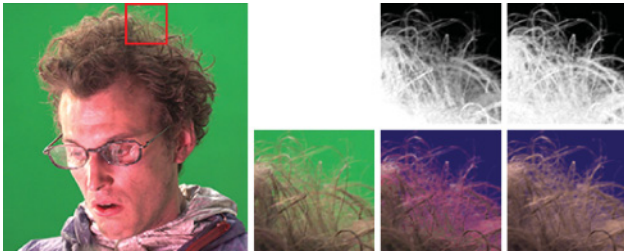
Fig. 2. High-quality alpha maps do not necessarily result in high-quality foreground layers for keying. While both alpha maps capture the intricate details of the actor's hair, the foreground layer computed by comprehensive sampling [Shahrian et al. 2013] (left) has noticeable color artifacts, while the foreground layer computed by our method has the correct colors.
