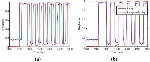
**Figure 6:** Two brightness signals over time. In (a) the offset between the signals is clearly visible, about 100 ms. In (b) the offset has been calculated and removed from the signals with the method discussed in Section 5.1.
