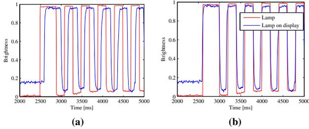
**Figure 6:** Two brightness signals over time. In (a) the offset between the signals is clearly visible, about 100 ms. In (b) the offset has been calculated and removed from the signals with the method discussed in Section 5.1.
