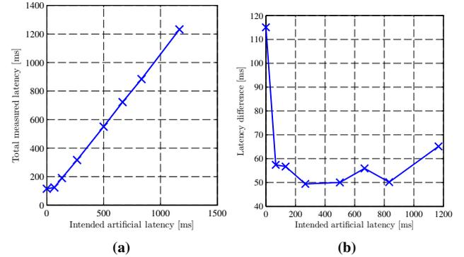
**Figure 7:** (a) depicts the total measured latency over the intended AAL. (b) shows the native latency (i.e. the difference between the total measured latency and the intended AAL) over the intended AAL.
