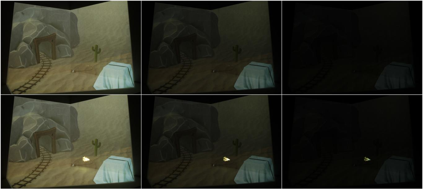
Fig. 9: Captured image of a sample projection mapped frame of a video sequence projected onto the three-sided mockup geometry. Upper row: Projection of the video projector alone. Lower row: Combined, geometrically, and photometrically registered projection using the video projector and GLP. Note the color hue correction as well as the significant local brightness variation. The exposure times are from left to right: 1200ms, 300ms, 75ms.
