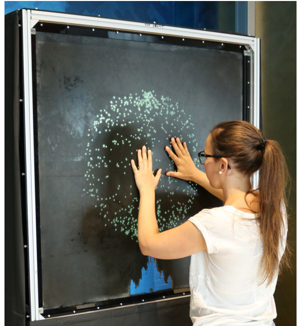
Figure 1. Feeling Fireworks is a large-scale tactile display which generates a tactile firework show, providing an extra dimension for blind and visually impaired users in the context of a universal experience that is shared by all.
