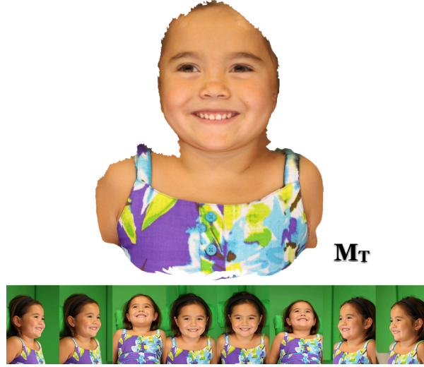
Figure 4: Example of a customer’s 3D facial scan ( M_T ). The 3D scanner presented by Beeler and colleagues [2] was used to acquire the data. The scanner utilizes the images shown in the bottom row to reconstruct the 3D geometry and colour.
