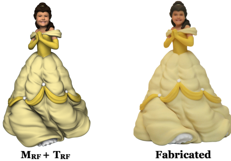
Figure 9: The system fabricates the completed customised figurine ( M_{RF} ) with a customised texture map ( T_{RF} ) using a colour 3D printer. We use a ZPrinter ® 650.
