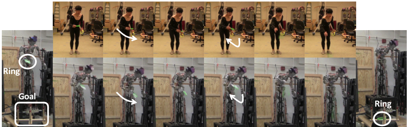
Fig. 10. Top row: the sequence of the player's demonstration. Bottom row: the sequence of robot motion mimicking that player's style. Player C tends to take the ring back slowly and largely, and throw from the side position. His bending tends to be deep. These features are imitated by the robot as shown in the picture.
