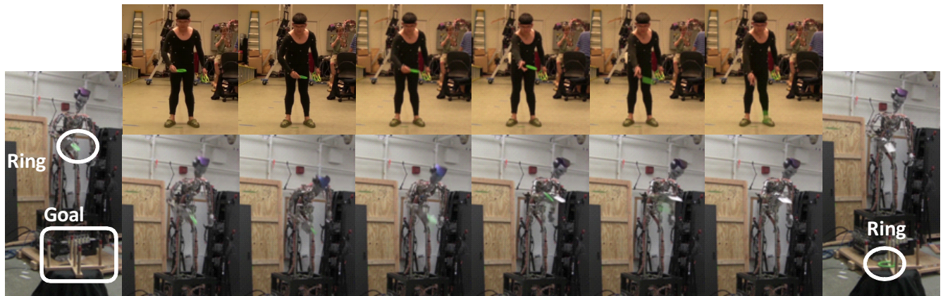
Fig. 9. Top row: the sequence of the player's demonstration. Bottom row: the sequence of robot motion mimicking that player's style. Player B tends to take the ring back lower, and toss the ring in the front. His bending is relatively deeper than first player, and his hand position during RELEASE task tends to be lower. Although the robot seems to bend excessively, probably to satisfy the required flying distance of the ring within the joint constraints, features described above are imitated by the robot.
