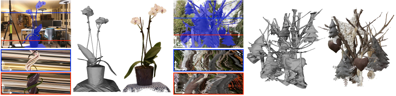
Fig. 1: Example results of our method captured with a rotating (left) and a hand-held (right) camera. Slices of densely sampled light fields reveal continuous structures that arise as a result of motion parallax (blue and red rectangles). Our method leverages the coherency in this data to accurately segment the foreground object in both 2D (blue image mask) and 3D (mesh), which can be used to aid 3D reconstruction algorithms (colored point clouds).
