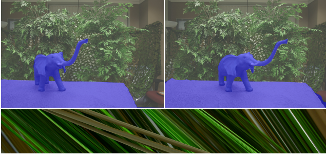
Fig. 8: Top: Our procedure applied to a linear light field from the USC/MERL light field repository to segment the foreground object. Bottom: One x - z slice of the light field demonstrating the motions of pixels.
