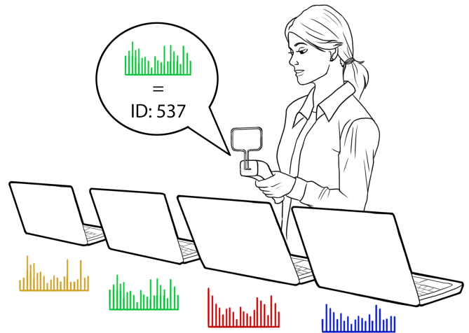
Fig. 1. Depiction of an IT professional scanning the unique electromagnetic noise generated by the unmodified laptops in order to determine their unique IDs and recover their asset management information.
