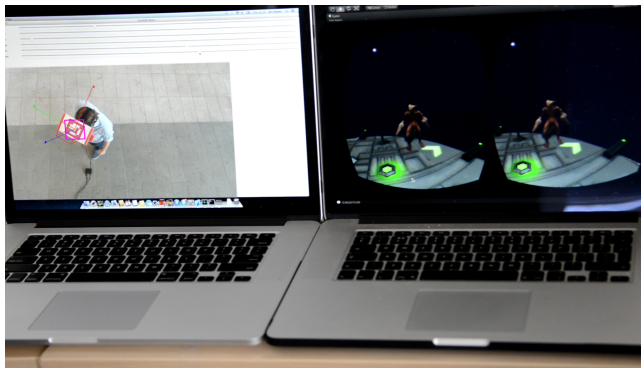
Figure 1: The server (left) processes camera data and sends it to the client (right) where it is filtered with the accelerometer data.
