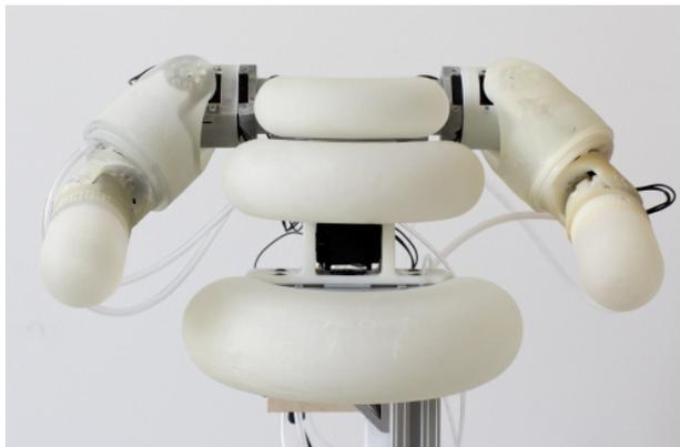
Fig. 1. Developed robotic upper body system with 3D printed soft skin modules. Our goal is the realization of a robot that can safely and playfully physically interact with children.
