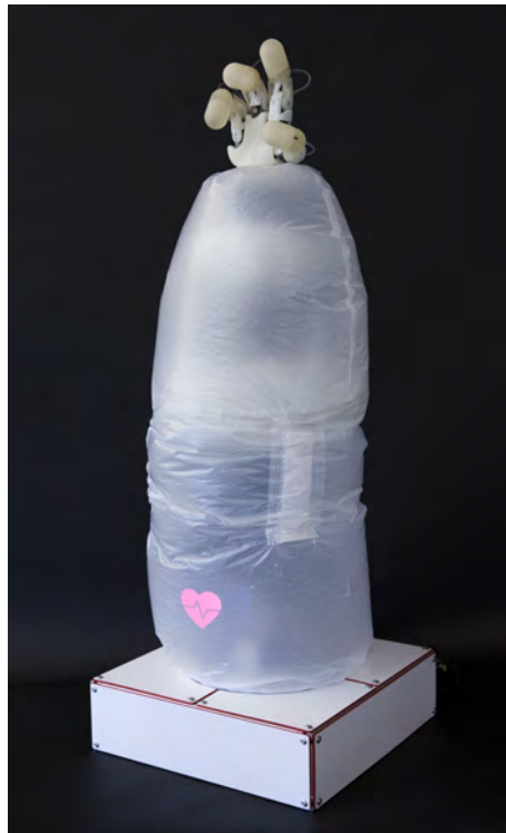
Fig. 1. Soft robotic arm system with inflated outer cover, underlying pressurized force sensing modules and soft 3D printed hand. Our goal is the realization of a robot that can safely and robustly physically interact with people.
