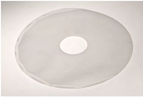
Fig. 4. The soft membranes of the force sensing modules on the arm are made of two laser-cut polyurethane circles heat-sealed around the outside edge. This image shows a partially sealed membrane during module fabrication. The left half of the membrane is heat-sealed
