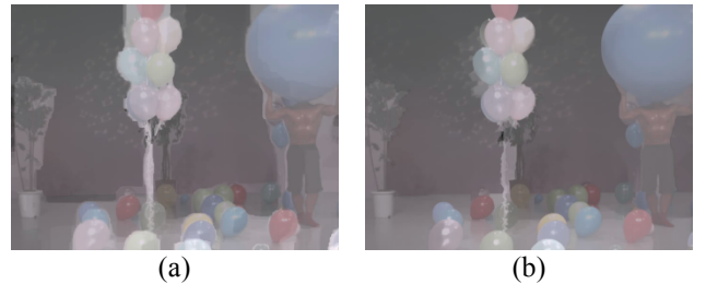
Fig. 1. Images overlaid with associated depth maps: (a) from MPEG’s 3D test data set, and (b) estimated with the Feature Flow algorithm. Note the strong alignment of depth edges with texture edges in (b).
