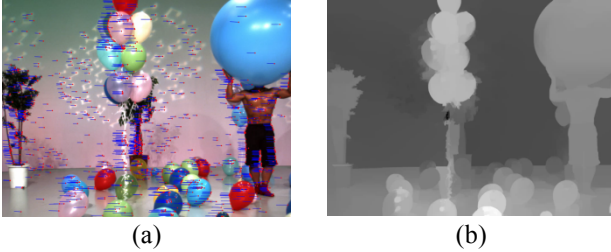
Fig. 2. (a) Sparse depth estimates, and (b) diffused depth map.
