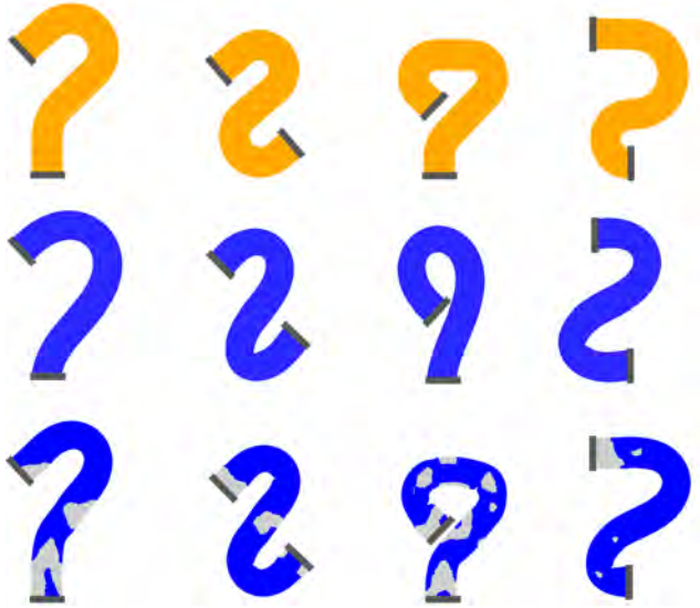
Figure 9: A straight bar is deformed into four different question mark shapes by imposing position constraints on its end caps. The first row shows the target shapes, the second row the result without material optimization and the third our results after material optimization (stiff/soft material shown in grey/blue color).
