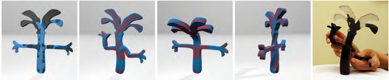
Figure 10: “Palmy3D.” From left to right: Rest pose with optimized material distribution (black/stiff, blue/soft), simulated poses (blue) overlaid with input target poses (red), 3D printed character.
