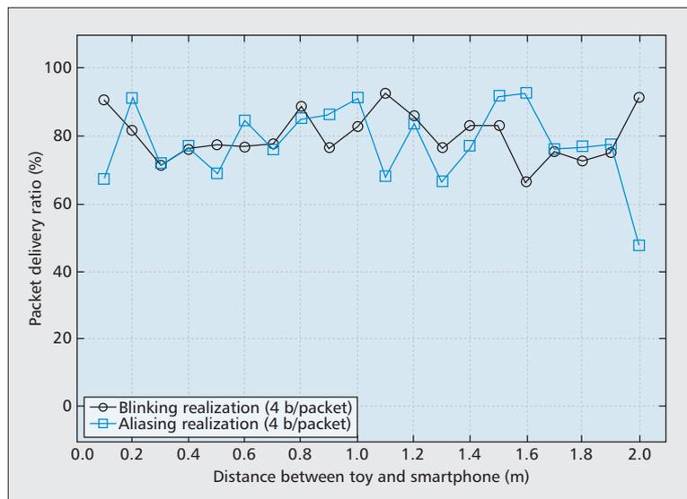
**Figure 5.** LED-to-smartphone communication mode: PDR over distance for an LED communicating to a camera; throughput: up to 1 b/s. Results are shown for distances of up to 1.5 m. The measurements result in the same packet loss ratio for both methods. However, the throughput is lower for the aliasing method because of the lower data rate (0.5 b/s and 1 b/s, respectively).
