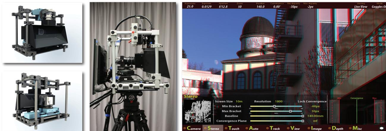
**Figure 1:** Our custom beam-splitter stereo-camera design is comprised of motorized lenses, interaxial distance and convergence. A programmable high performance computational unit controls the motors. User input is performed using a stereoscopic touch screen.
