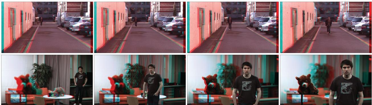
**Figure 9:** Two examples of automatic control based on template tracking. Manual interaction is only required in the first frame (left column) to initialize the subject of interest. In the top row, the controller follows the convergence plane at the depth of the subject. In the bottom row, both convergence and focus are following the subject.
