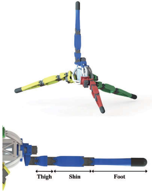
Fig. 15. A spherically symmetric quadruped robot, Tetrabot. (Top) The zero pose of Tetrabot is similar to a tetrahedron. (Bottom) Each leg has 4 DoFs including one yaw joint and three pitch joints.
