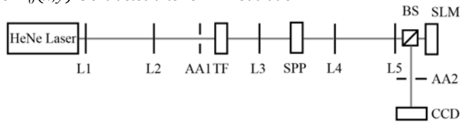
Fig. 2. Schematic overview of encoding and decoding a two-dimensional image with OAM, where L1 to L5 are the lenses, AA1 and AA2 are the adjustable apertures, TF is the transparency film, SPP is the spiral phase plate, BS is the beam splitter, and SLM is the spatial light modulator.
