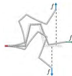
replace a segment of a straight rod with an instance of a template, and apply forces to one end while holding the other one fixed (see inset), we observe a highly heterogeneous, anisotropic, and force-dependent behavior: if we apply an upward-pointing force (in blue), and apply the same force with opposite sign, we see an asymmetric deformation. If
