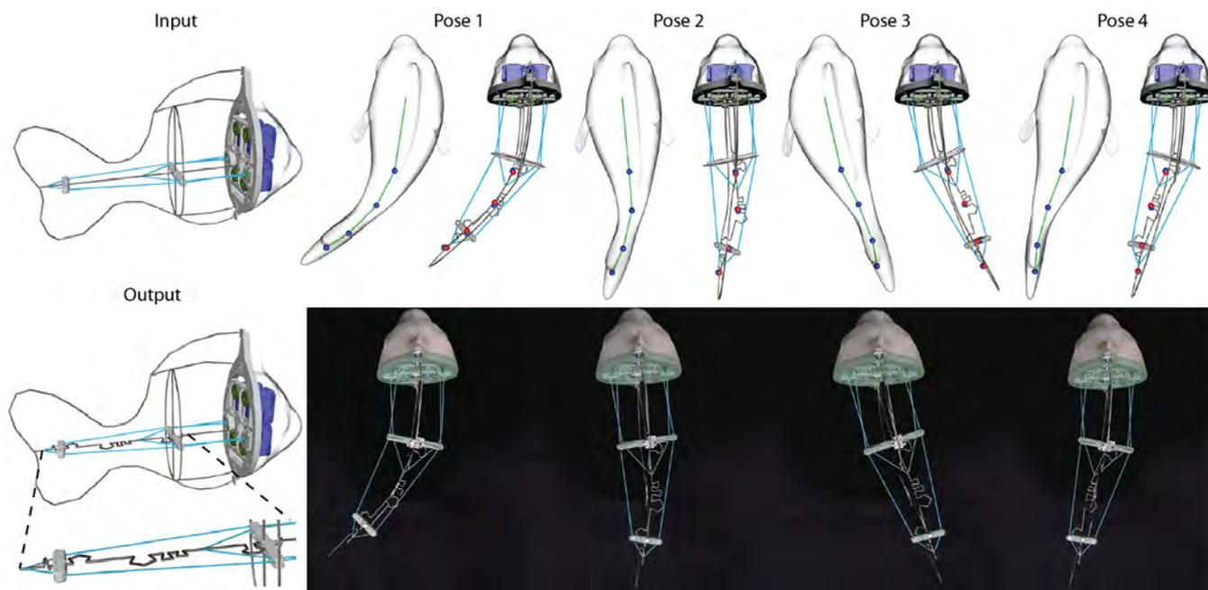
Fig. 18. **Animatronic Fish.** The input and optimized wire structure (on spine) are shown on the left from the side view. The first row also shows the 4 target poses (top view), from the input animation driven by the skeleton (in green) and output animation driven by the cables on the spine. The second row presents the frames for the swimming fabricated fish. The deformations are large and nonlinear.
