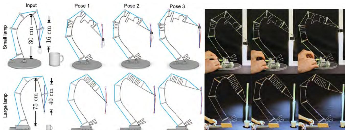
Fig. 17. **Compliant Lamps.** Using wire of 2 and 4 mm diameter respectively, we designed and fabricated a small and a large lamp. Closely matching the targeted linear trajectories (in blue), we compensate for the self-weight of the wire and the weight of the attached light bulb.
