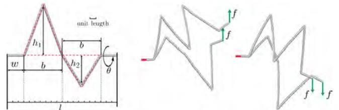
Fig. 8. **Generic Template.** Keeping the length  $l$  and triangles’ base  $b$  constant, our four-parameter template (left) fulfills our desiderata of genericity. Asymmetric configurations allow us to control the anisotropy and magnitude of the homogenized bending stiffness (right).
