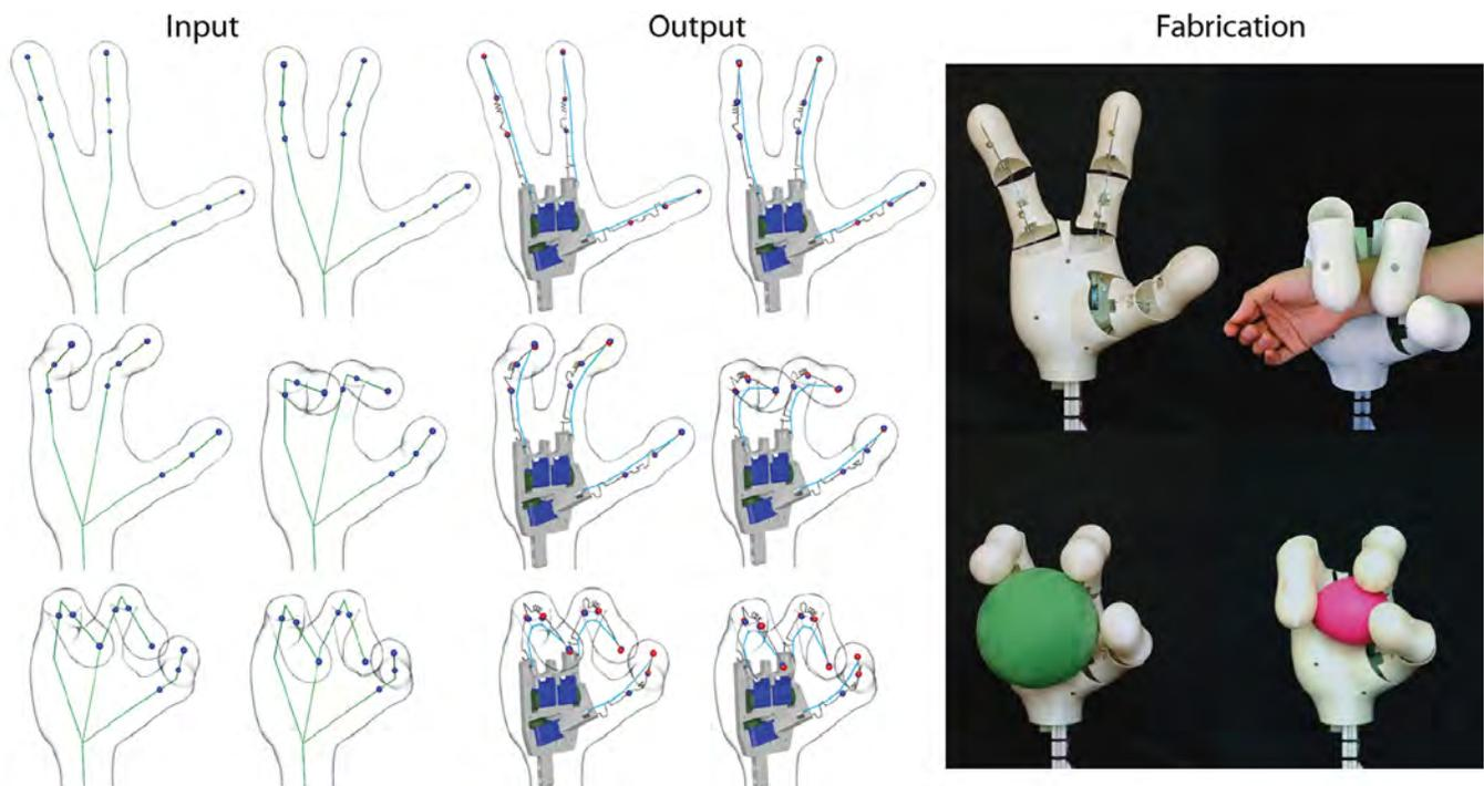
Fig. 15. **Robotic Alien Hand.** We turn a grasping animation (Input) of a hand with three fingers into a lightweight, compliant robotic hand (Output). We match corresponding targets (in blue) from 5 keyframes well (in red). Interactions with the hand are safe as we illustrate with grasping an arm and fragile objects like balloons of different sizes.
