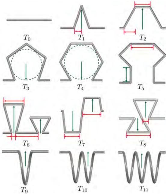
Fig. 6. **Fabricable Templates.** Besides the straight rod  $T_0$ , we support polygonal templates ( $T_1$ - $T_5$ ) which become more compliant with increasing number of sides. Our twin templates ( $T_6$ - $T_8$ ) consist of two isosceles trapezoids and further increase the stiffness gamut. Our helical springs ( $T_9$ - $T_{11}$ ) are not directly fabricable on the bending machine but are compact. Red parameters remain fixed when we fine-tune the green parameters.
