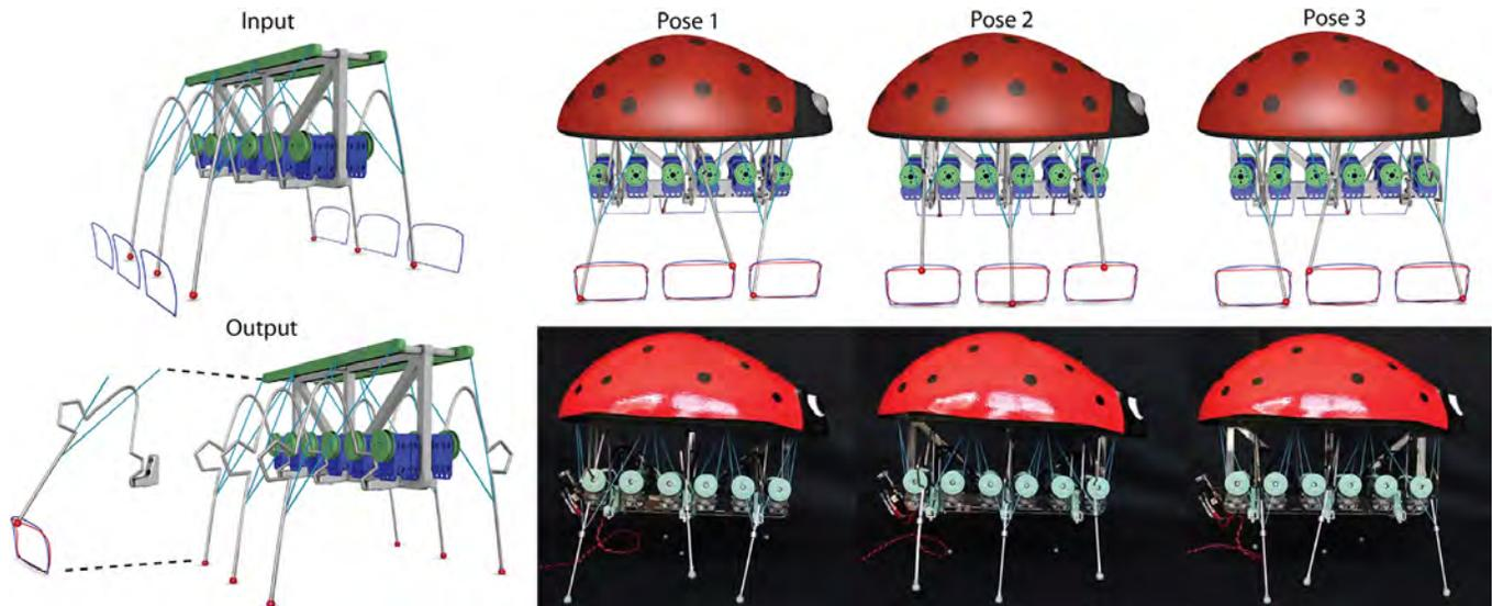
Fig. 14. **Walking Ladybug.** We optimized a spline-specified, curved leg (Input) to perform a desired end effector trajectory when actuated with two cables (Output, compare red and blue trajectories). Visualizing simulations for 3 out of 8 trajectory samples (Pose 1-3), we observe excellent target matching performance. We compensate for the self-weight of the robot and contact with the ground during our three-stage optimization, resulting in a stably walking robot.
