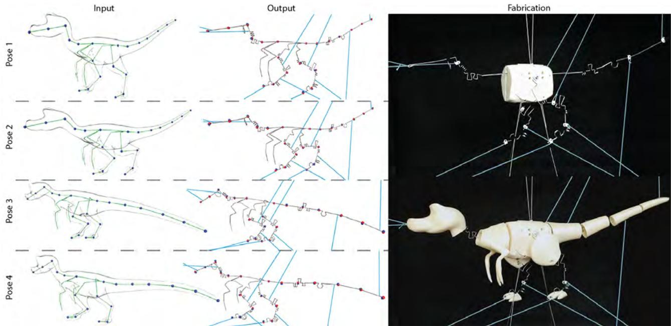
Fig. 13. **Kinetic Dinosaur.** We extract 4 keyframes from a walking cycle of a rigged dinosaur (Input, left column), matching corresponding target points (Output, middle column, in blue) on the animated rig by co-optimizing the wire's rest shape (red markers) and cable forces. The fabricated character with (bottom) and without (top) lightweight, 3D printed shells is shown in the right column.
