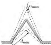
As will be discussed in Sec. 5, fabricable shapes are limited by a maximum bending angle  $\alpha_{max}$  and a minimum distance  $d_{min}$  between discrete bends, as shown in the inset on the left. Note that these fabrication constraints are universal. However, when switching devices or the wire, their values change.
