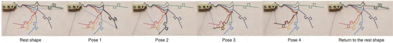
Fig. 12. **Validation.** A physical finger pulled on with optimized cable forces matches simulations closely (shown on the background paper with 5 mm grid spacing). Even after large deformations (target in red), our optimized kinetic finger does not plastically deform (Rest shape vs. Return to rest shape). Images are taken from a single continuous video sequence, which is included in the accompanying video.
