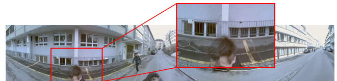
Fig. 19. Failure case: ghosting effect of an object too close to the camera array.
