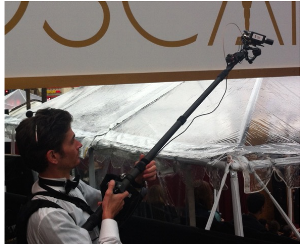
Figure 1: A lightweight camera on a 3dof active gimbal and boom is susceptible to vertical disturbances.
