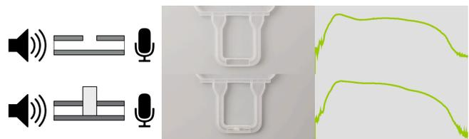
Figure 5. Open (top) and blocked tubes.
