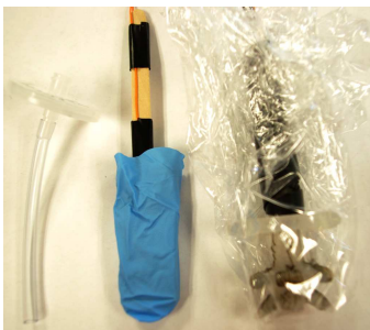
Figure 2: All three devices, ready for testing. From left to right: sip/puff mouthpiece, bite sensor, and tongue joystick. Four-direction selection is accomplished using the actions in the table.
