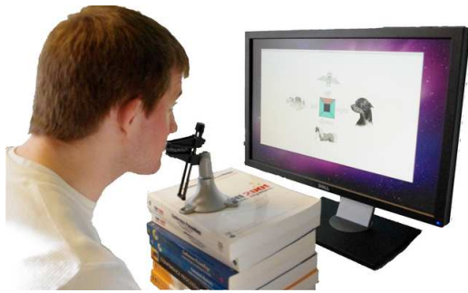
Figure 6: A subject performs a forced-choice four-direction speed test of the tongue joystick.
