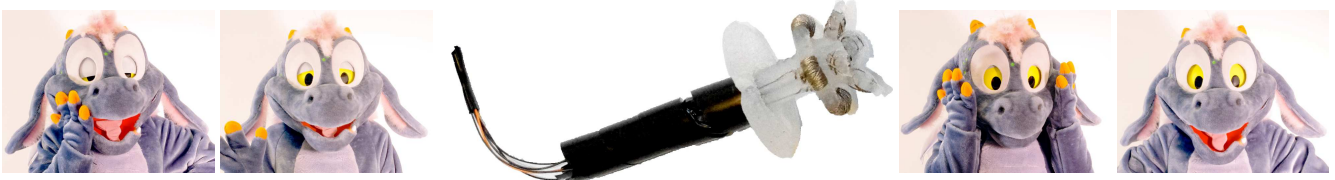
Figure 1: Our tongue joystick allows an actor to invisibly select prerecorded audio clips, letting the articulated-head dragon converse with children in its own voice.
